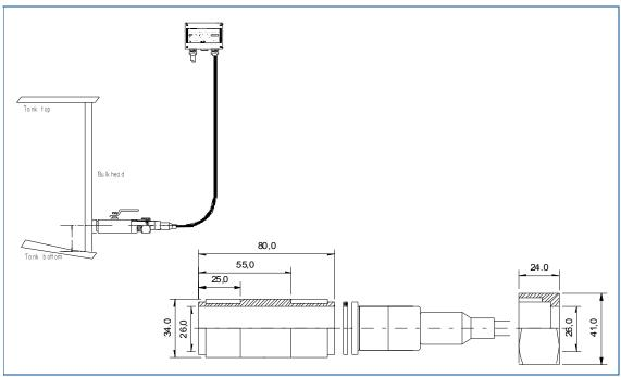
The thread collar and the nut are manufactured of SS 316L steel. The gaskets are made of nitrile rubber
